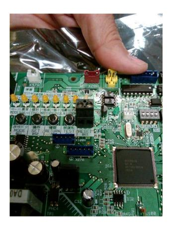
3) Hunt Engineering designed an automatic restart controller with timing relays to mimic the operation of the manual push button we replaced.
